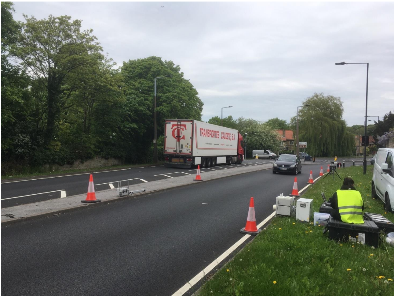
Figure 3 Photograph of the OPUS instrument set-up on the A635 Westbound.
